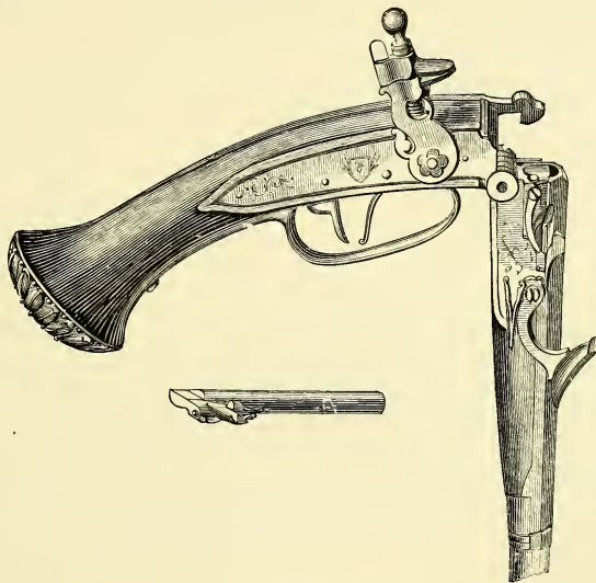
Early Breech-loading Flint-lock Pistol.
